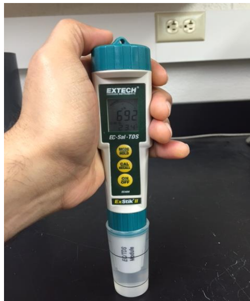
Figure 3.15. Measuring pore-water resistivity using Extech-400 conductivity meter
