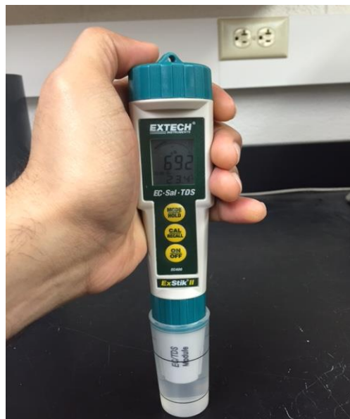
Figure 6.13. The Extech 400 conductivity meter in use
