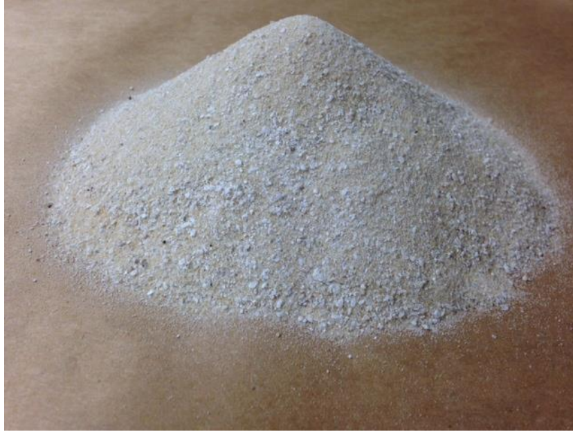
Figure 4.1 Soil M30 (sand with 30 % gypsum)
